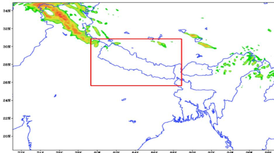
**Figure 1: An example of double nested domain stetting for new DHM system. Grid size in outer and inner domains could be 9 and 3 km, respectively.**
