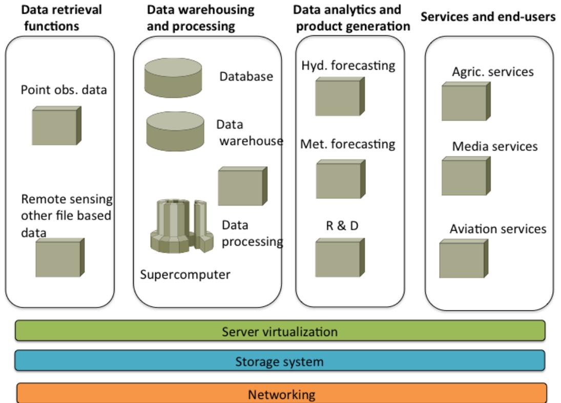
**Figure 2. Production system functions and supporting ICT systems**
