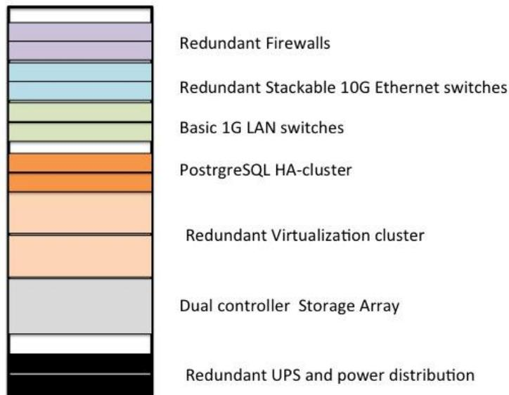
**Figure 5. Data Center Rack layout**
